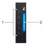
Figure 14. Left control panel without optional iDRAC Quick Sync 2.0 indicator
