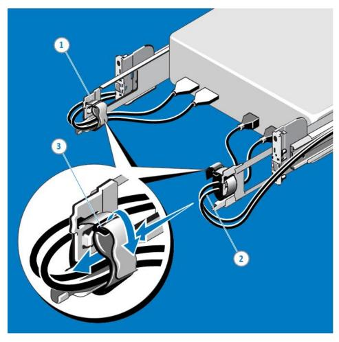
Figure 58. Routing the Cables
