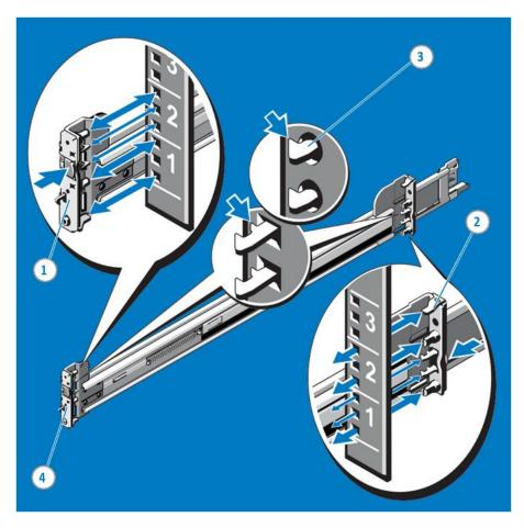
Figure 53. Installing and Removing Tool-Less Rails
