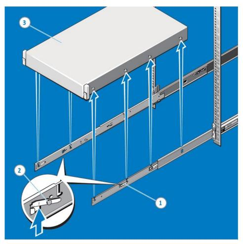
Figure 56. Removing System from the Rack
