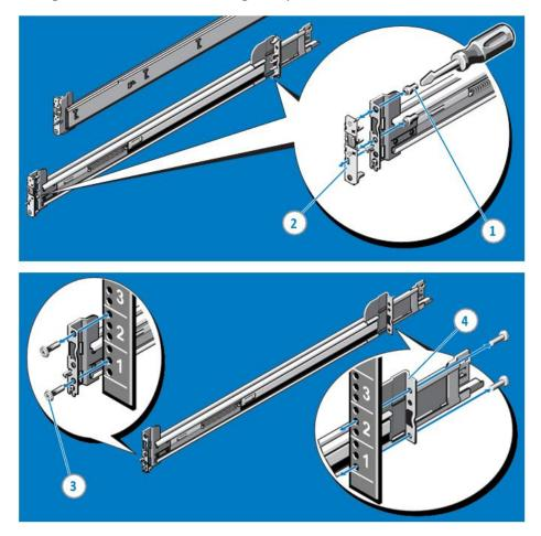
Figure 54. Installing and Removing Tooled Rails
