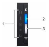
Figure 25. Left control panel with optional iDRAC Quick Sync 2.0 indicator
