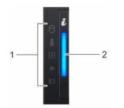
Figure 3. Left Control Panel without optional iDRAC Quick Sync 2.0 indicator
